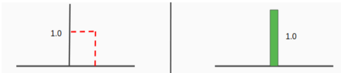
Fig 5.2 Impulse function in discrete world and continuous world
